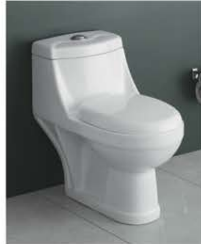
TRISTA (wash down) L 715 W 380 H 665mm S-Trap 220/300mm P-Trap 180mm
