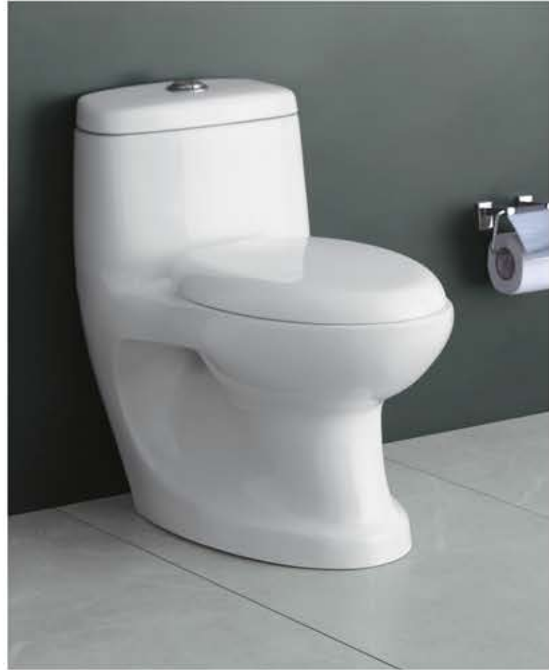
SISTO (wash down) L 715 W 390 H 705mm S-Trap 95/230/300mm P-Trap 180mm
