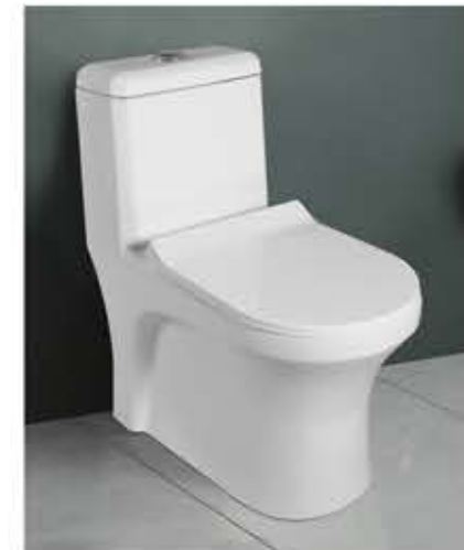
TERZO (wash down & Siphonic) L 660 W 355 H 735mm S-Trap 240mm (Wash Down) S-Trap 300mm (Siphonic) P-Trap 180mm
